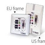
**EFI-6700** - Standard model with infrastructure LAN integration capability. This model has generous number of USB ports for improved connectivity and offers True Color display support. Owns built-in Power-over-Ethernet capability in addition to external powering.
